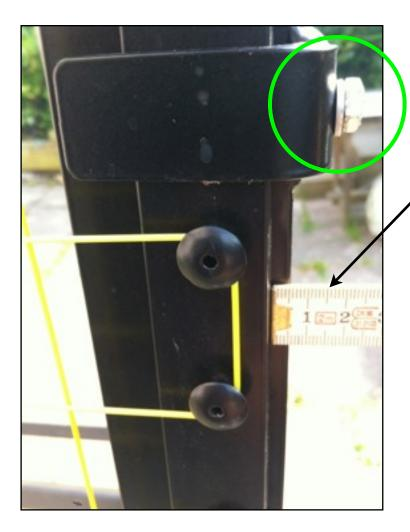
Tighten the screws (**green circle**) on the adjustable list after having merged the entire horizontal string with the vertical string and fixed the knot in the bottom right side of the frame.
