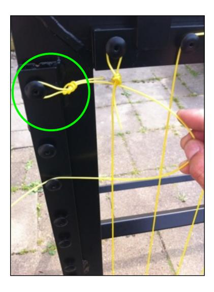
Fix the knot at the end of the string on the knot in the top left corner of m-station, as illustrated on the picture.
