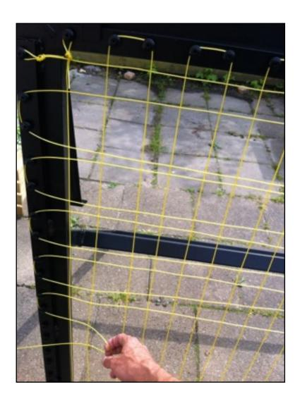
Keep going until you have merged all the horizontal strings with the vertical strings and pulled the strings around the fixed points on the left and on the right side of the frame.
